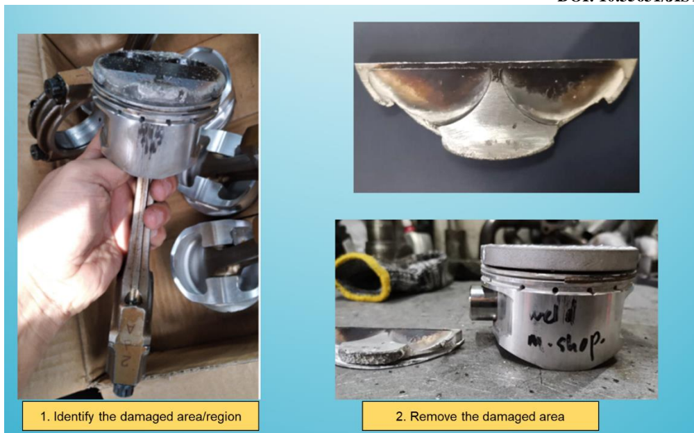
Figure 3: Inspection of Damaged Area and Part Pre-Processing
