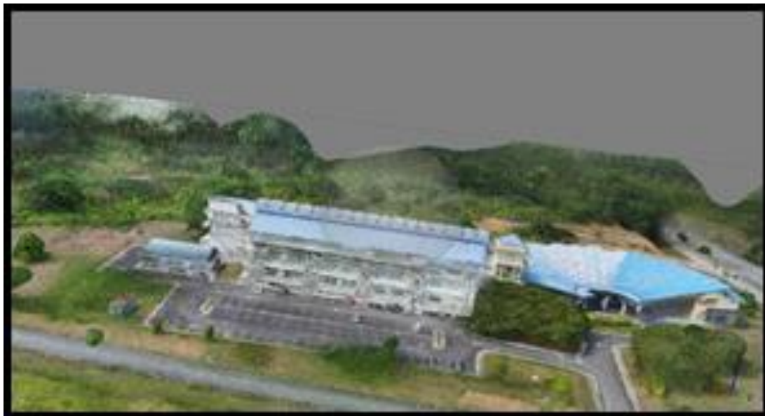
Figure 5: The 3D Building Model Based on Nadir and Oblique Aerial Images.
