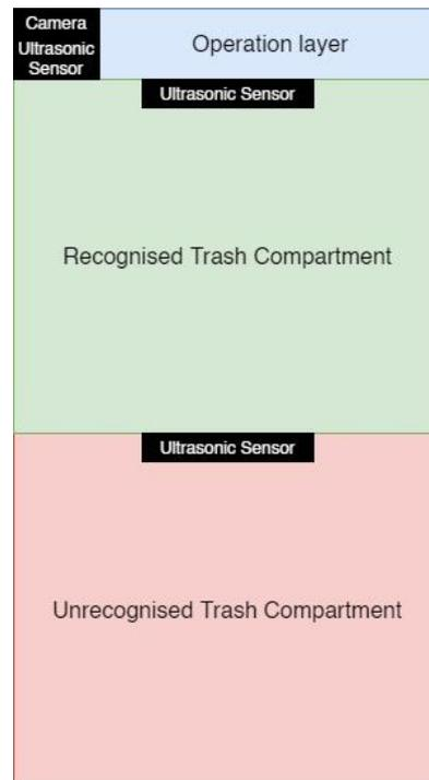
**Figure 5: Basic Architecture Diagram of the Smart Bin**
